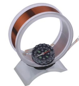
Demonstrator of Left and Right Hand Rules Art No: EMT04002
