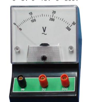
Voltmeter, AC Art No: VLT009 Measuring Range: 0~30V 0~300V
