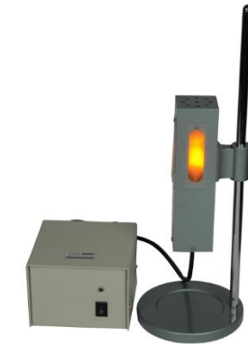
Sodium Lamp with Power
