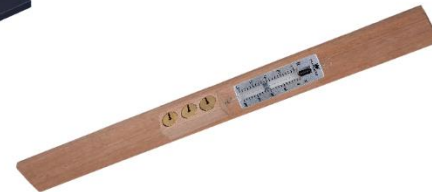
Friction Apparatus Art No: DY08002 With 3-50g weights & a 100g spring scale.
